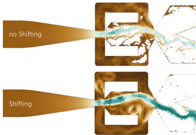
Shifting enforces a homogenous particle distribution by applying a diffusion term. This increases the simulation quality significantly.
