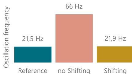
In comparison with experimental reference data, the effect of shifting becomes clear: the oscillation frequency is now accurately predicted.
