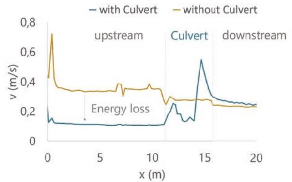
*Comparison of flow velocities with and without culvert*
