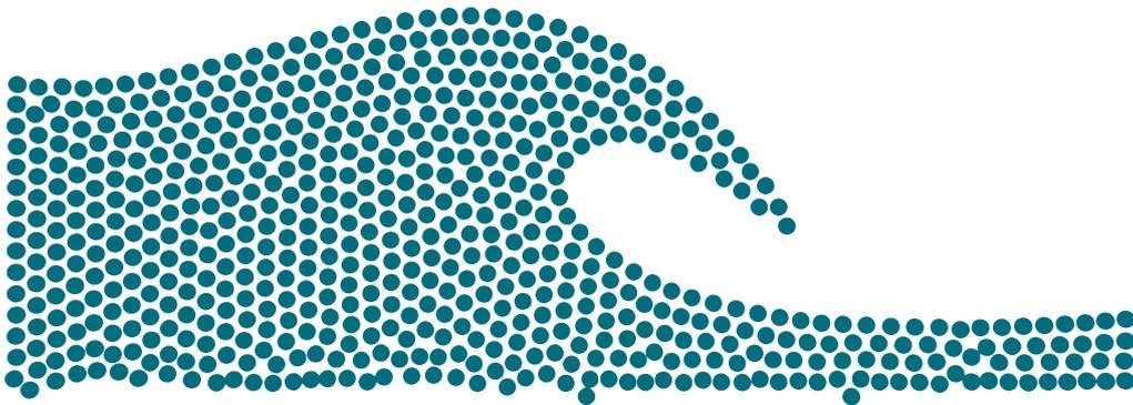
*New particle-based fluid model (SPH)*
